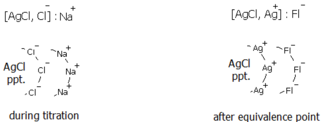
Figure 7-2 Fajan's Method for the Titration of Chloride
